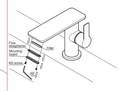
If the flow rate gradually decreases after sometime, it usually results from poor water quality leading to blockage of the filter. Please clean the filter as shown in figure above: Turn off the handle, unscrew the M3 screw with the S2 spanner, take off the mounting board, the flow straightener and the filterin turn, wash the filter and then install them back.
