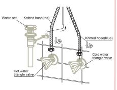
Connect the two knitted hoses to the two triangle valves (Red for hot water and blue for cold water).
