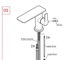
Connect the upper lift rod with the lower lift rod.Insert the lift nut into the slot on the back of the mixer body and connect it with the upper lift rod. Screw the knitted hose with red(hot) in front and bule(cold) in back.
