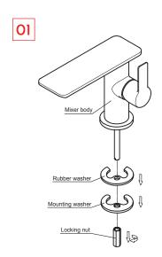
Disassemble the locking nut, mounting washer and rubber washer from the mixer body in turn.
